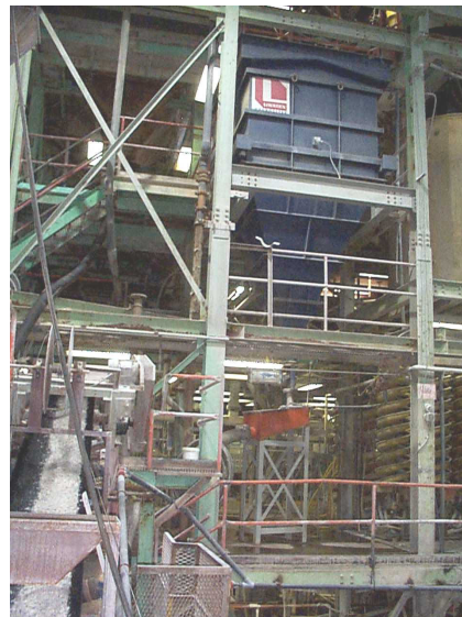
Figure 2. Linatex hydrosizer (blue)
